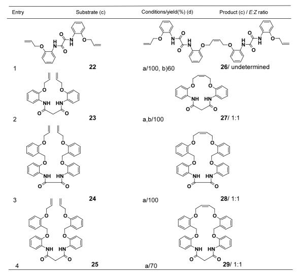
a) Substrate (0.01 M), Grubbs' catalyst I (2.5 mol%);  $CH_2CI_2$ , reflux 2 h, b) Substrate (0.01 M), Grubbs' catalyst I (1 mol%);  $CH_2CI_2$ , reflux 6 h, c) All substrates and products were analyzed by <sup>1</sup>H, <sup>13</sup>C NMR, GC-MS, and gave satisfactory elemental analyses, d) The yields were determined by 400 MHz <sup>1</sup>H NMR.<sup>24</sup>
